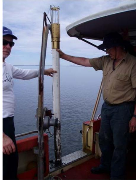
Figure 2. Collection of cores (80 mm diameter PVC).
